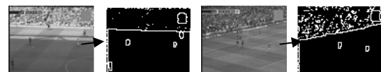
Figure 6. Two sample of the result of applying Laplasi Filter to the output of grass detection phase.
